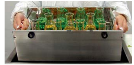
The removable shaking insert prevents direct contact with the bath fluid. Carrier trays can be assembled comfortably outside the bath.
