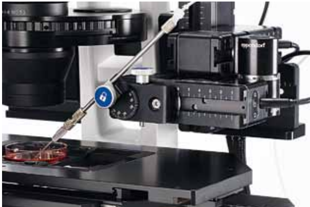
InjectMan 4 micromanipulator mounted for axial injection.
