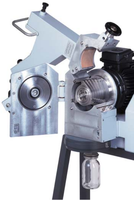
View into the fold-back housing of the SM 2000 with collecting unit for wide mouth bottles
