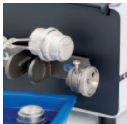
Before grinding takes place the grinding jars are immersed in liquid nitrogen (-196 °C) in the cryo box for approx. 2 - 3 minutes
