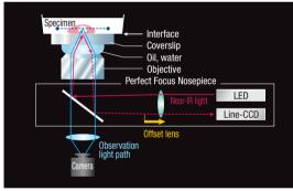
The diagram shows the case when an immersion type objective is used. A dry type objective is also available
