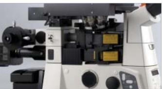
Example: In addition to the PFS, a photo activation module (upper tier) and a back port (lower tier) are mounted.
