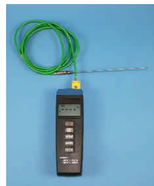
MIN/MAX digital thermometer with add. temperature sensor
