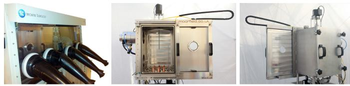
Left: MiniLab 090 system for LTE deposition fitted to 4-gloveport glovebox. Middle: MiniLab 090 chamber outside glovebox and with front door opened, revealing thermal evaporation sources inside. Right: Rear of MiniLab 090 chamber showing rear service door for easy access to chamber interior from outside glovebox.
