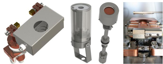
Above: Examples of deposition sources available for the MiniLab 090. From left to right: Moorfield TE1 source for standard thermal evaporation, Moorfield LTE-1CC source for low-temperature evaporation (LTE), Moorfield *Flexi-Head* MAGNETRON source for magnetron sputtering, and Telemark multi-pocket water-cooled electron-beam source.
