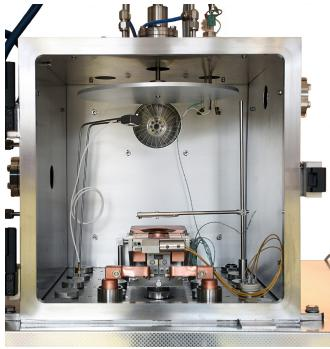
Above: Examples of MiniLab 060 chamber configurations. Left: Chamber fitted for thermal evaporation, with Moorfield 4-pocket TE4 thermal evaporation source. A quartz lamp array for substrate heating is also included in this system. Right: System equipped for electron-beam deposition, with Telemark source and  $6 \times 7$  CC pocket configuration. Both setups have substrate rotation and quartz crystal sensor heads for deposition rate/thickness monitoring/control.
