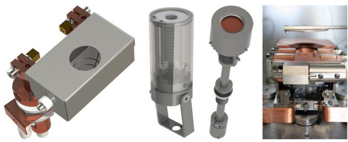
Above: Examples of deposition sources available for the MiniLab 060. From left to right: Moorfield TE1 source for standard thermal evaporation, Moorfield LTE-1CC source for low-temperature evaporation (LTE), Moorfield Flexi-Head MAGNETRON source for magnetron sputtering, and Telemark multi-pocket water-cooled electron-beam source.
