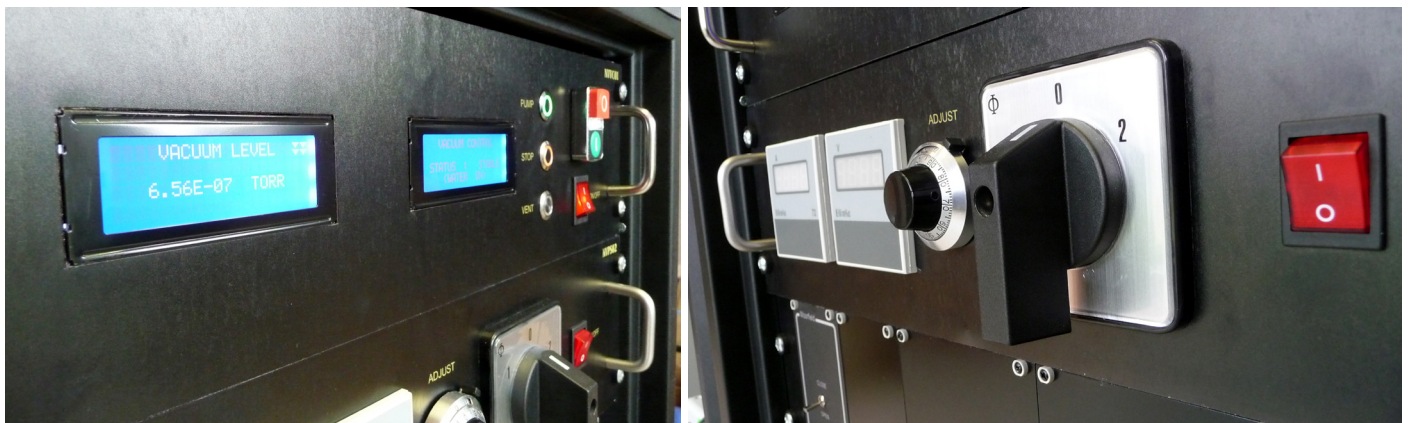
Above: M307 system control panels, mounted in the electronics rack included with the unit. Left: Vacuum monitoring and pump/vent control unit. Right: Thermal evaporation power supply and control unit (for system configured for thermal evaporation).
