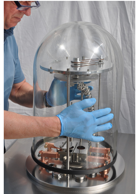
Above: Lifting off the M307 bell-jar to access in-chamber hardware.
