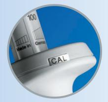
It can be readjusted when tested according GLP and calibrated for liquids with a different density than water. According to EN ISO 8655 the readjustment for more safety and transparency is sealed.
