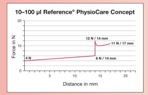
Optimized operating forces are important for the daily work routine in the lab. The low weight of the Eppendorf Reference<sup>®</sup> of 89 g resp. 99 g and our
