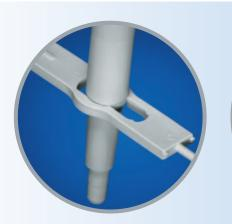
We give you the key to user-maintenance. With the universal wrench provided with the pipette, you can carry out small service tasks yourself.
