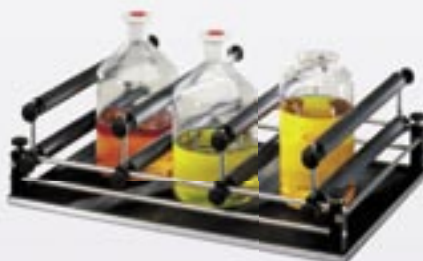
Rack System Combifix SM B No. 0050 155 Basic rack with 4 clamping strips h and 4 clamping strips v. For fastening horizontal vessels between the clamping strips, or as added support for high vessels. The maximum distance between the strips h and v is 60 mm. With additional strips also suitable for other vessels (see page 22).
