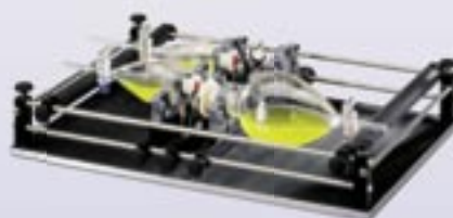
Rack System Combifix SM C No. 0050 156 Rack system with 2 clamping strips h, 2 cramp strips and 1 spring strip. For fastening separating funnels. Standard version of cramp strip: 5 clamps NS 19 (D20) and 2 clamps NS 29 (D32). With additional strips also suitable for other vessels (see page 22).
